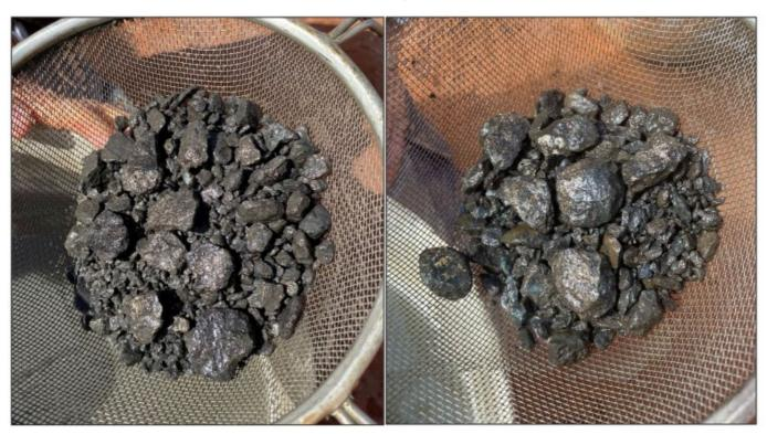
Figure 8: RC Drilling chips showing sulphide minerals from MMRC01 184-185m (left) and MMRC04 203-204m (right)
