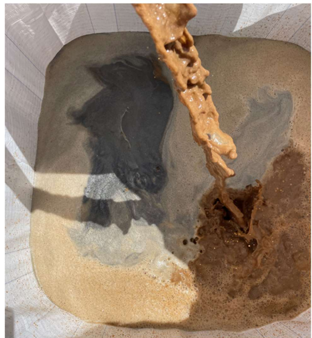
Figure 2 & 3: Spiral testwork underway at AML on the fine component of the sand material (left). Lower density cut from the spiral with visible graphite on the surface (right)
