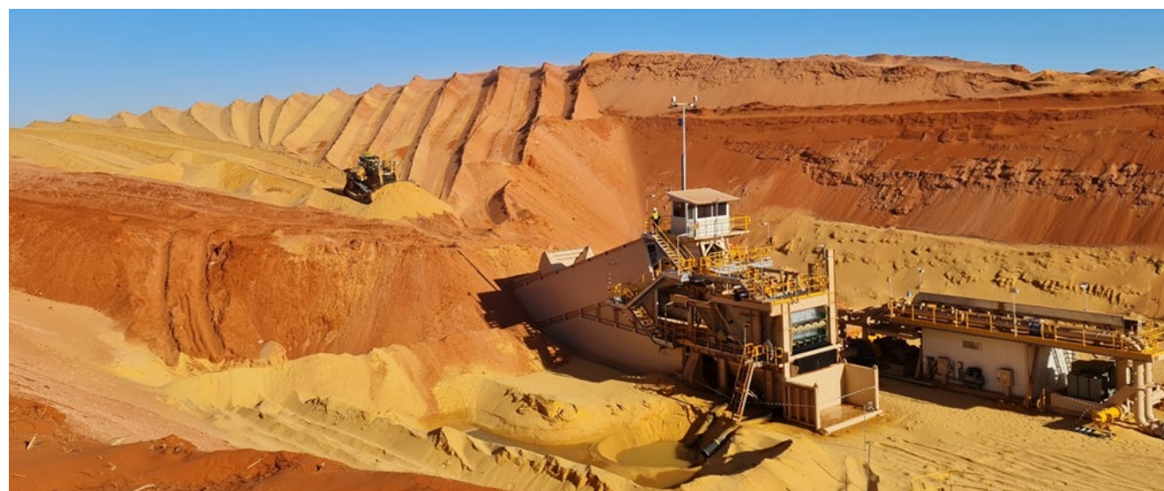
Figure 5 Coburn Project – Dozer Push Mining of Free-flowing Sand
