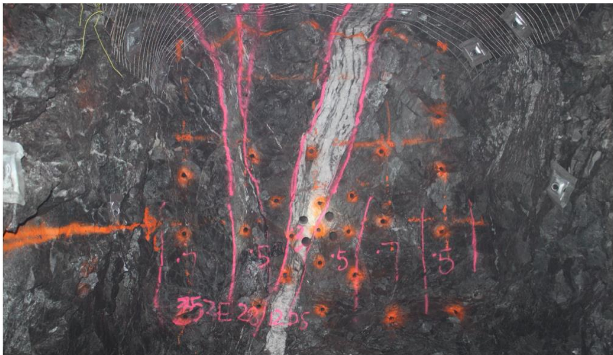
Image 3: 253 SOE level lowest in the mine vein grade 19.53 g/t Au
