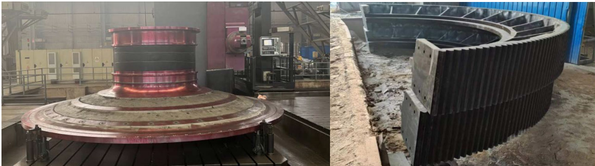
Figure 7: Mill end fabrication (left), Mill girth gear fabrication (right)
