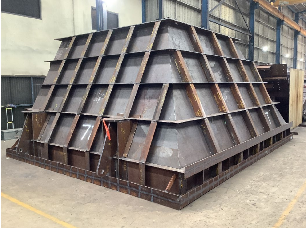
Figure 7: Mill end fabrication (left), Mill girth gear fabrication (right)
