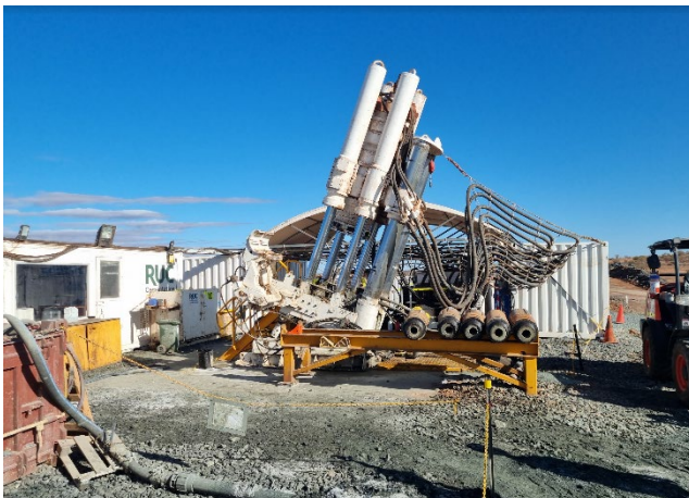
Figure 9: Bellevue site RUC raisebore drilling at the Northern escapeway rise (left); Second raisebore drilling rig at the Southern ventilation rise (right)
