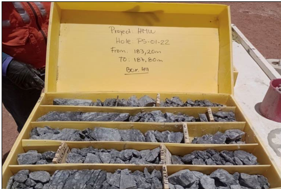
Figure 7 - Highly fractured rock core obtained from PS-01-22
