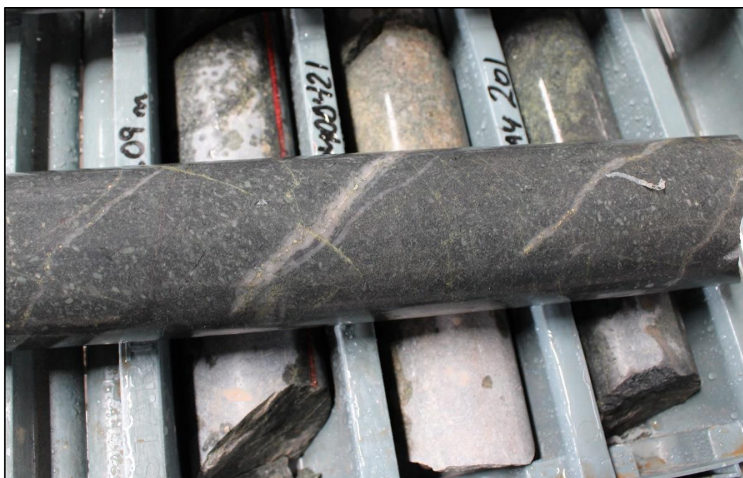
Figure 3. HQ diamond core from Corvette diamond hole 22MYDD421 at 817.5 metres, highlighting the abundance of early quartz veins with a centre-line of sulphides (also known as B-veins) crosscut by later epidote-chalcopyrite veins. This mineralisation forms part of a zone that grades 13 metres at 1.07% Cu & 0.61g/t Au (ASX MAG 30 January 2023).
