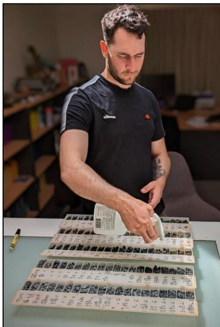
Field Technician recording portable XRF readings on REE drill chip tray samples.
