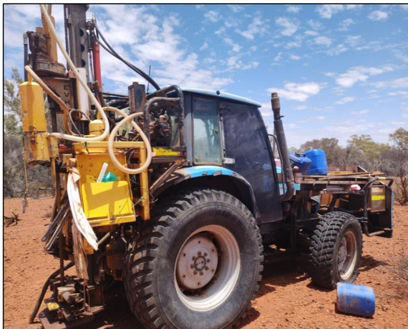
Vacuum drill Rig at the Ytria REE Prospect
