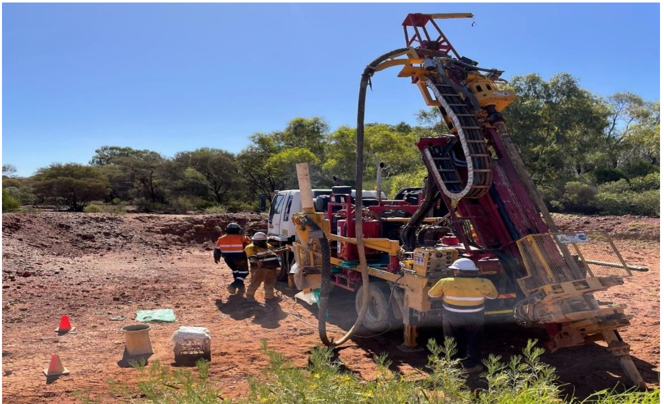
Aircore drill rig on site at Crown Prince gold prospect
