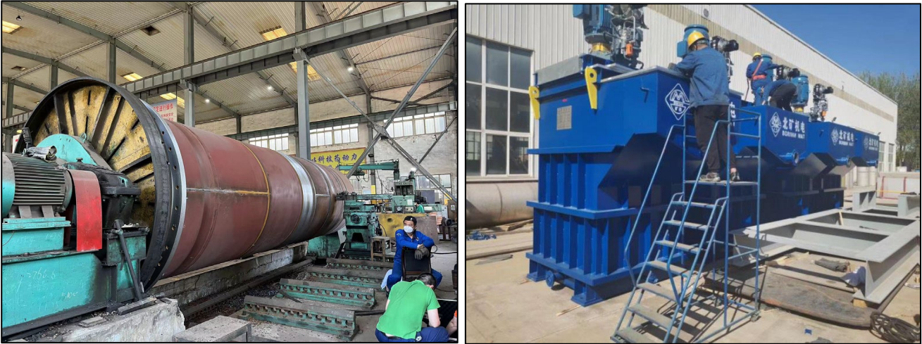
Figure 5: Inspection and testing of the rotary drier (left) and BGRIMM attritioning mills (right). The manufacturing, QAQC and factory acceptance testing is complete and the equipment in storage in China.
