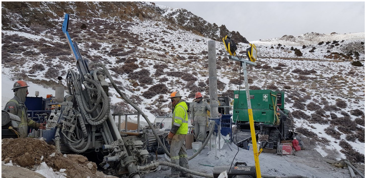
Figure 1. RC percussion drill rig on site drilling the first hole at Star Canyon, Nevada, December 2022.
