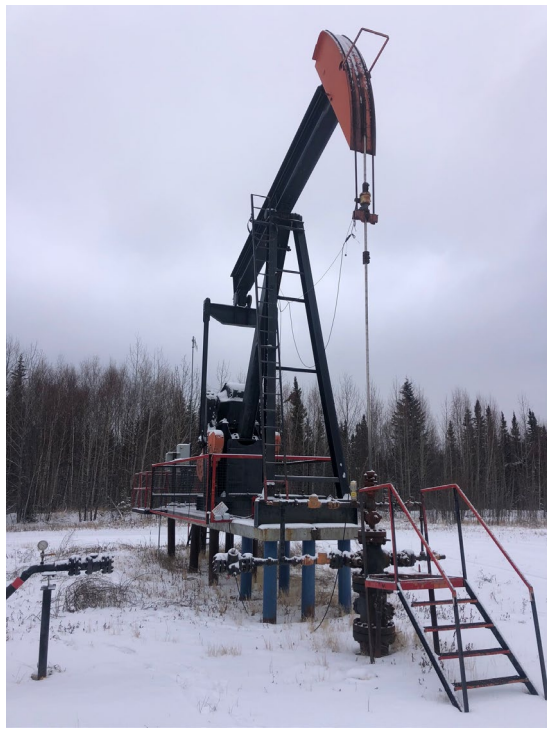
Pump jack at Red Earth
