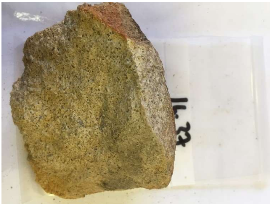
Figure 10 - Rock chip of outcropping from Figure 5 silicified caprock of fine brecciated quartz in a clay matrix
