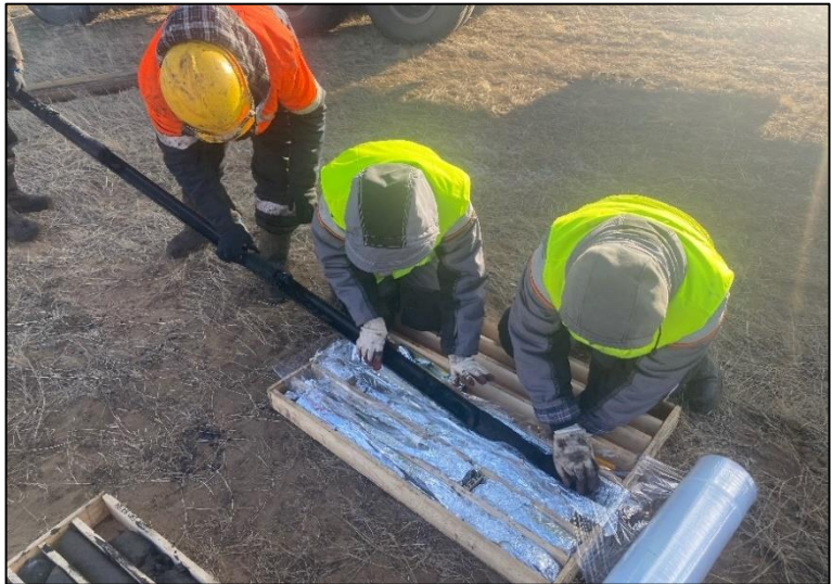
Figure 3. Rock and coal core collection from HQ DD drilling.
