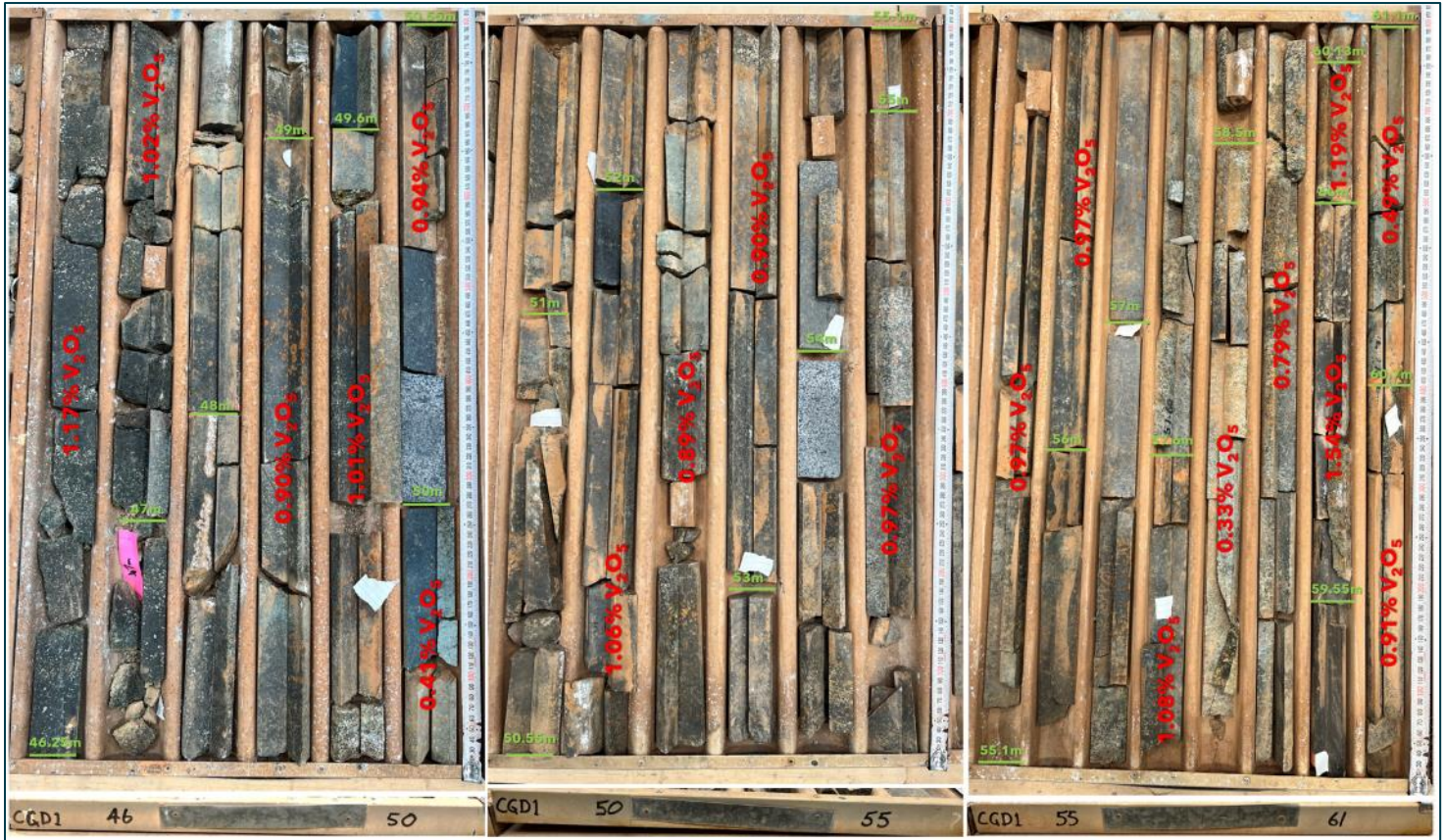
Figure 3; Drillhole CGD01 from 46.25m to 61.1m. Intercept totals 15.7m at 0.90% V 2 O 5 as part of a wider interval of 28m at 0.90% V 2 O 5 . Note massive magnetite observed in the drillhole which is characteristic of high grade VTM mineralisation.
