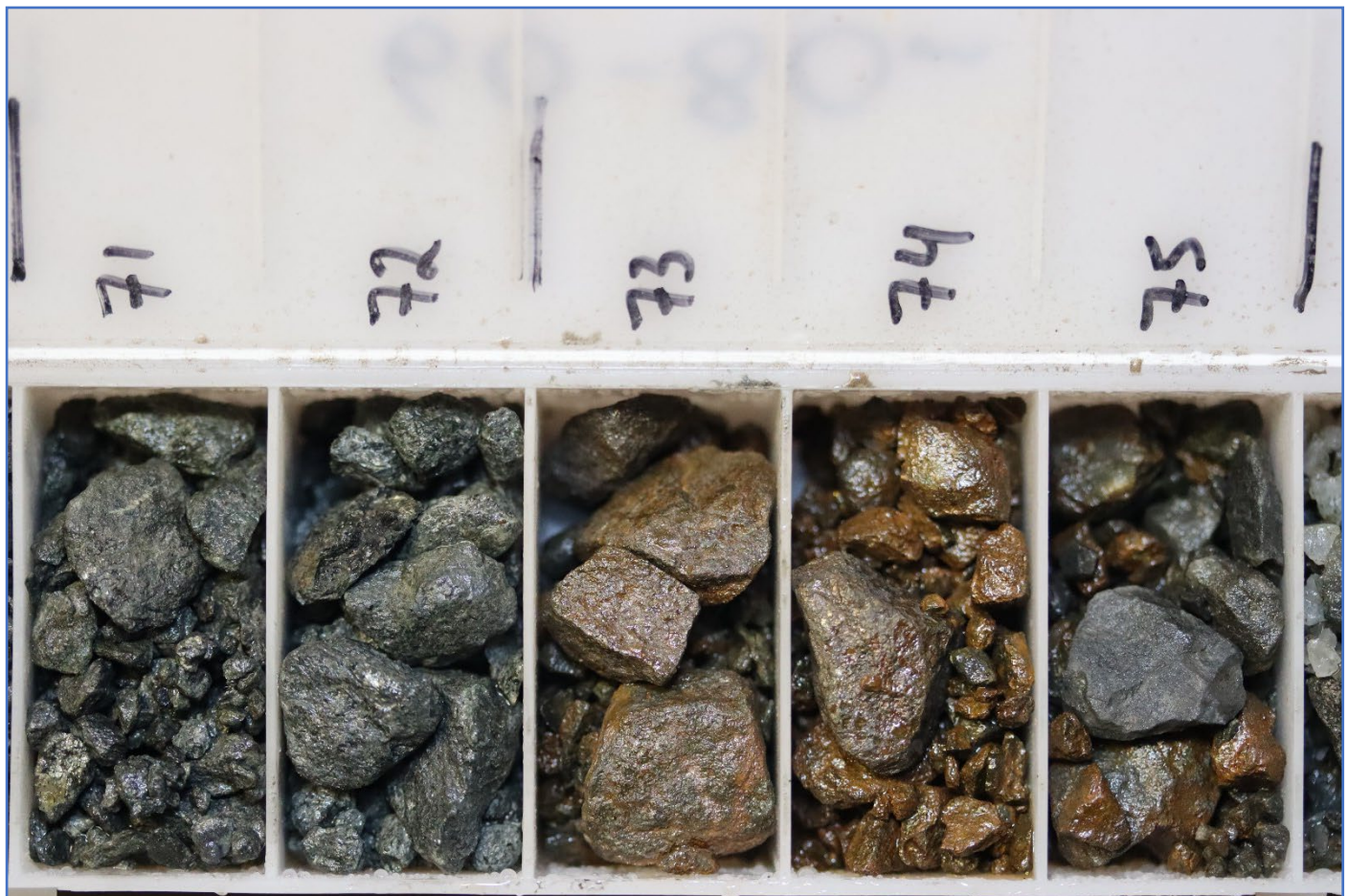
Figure 5: Visually logged chips from 23NRC011 showing massive pyrrhotite with minor chalcopyrite from 72-74m with some of same mineralisation extending into the next metre *
