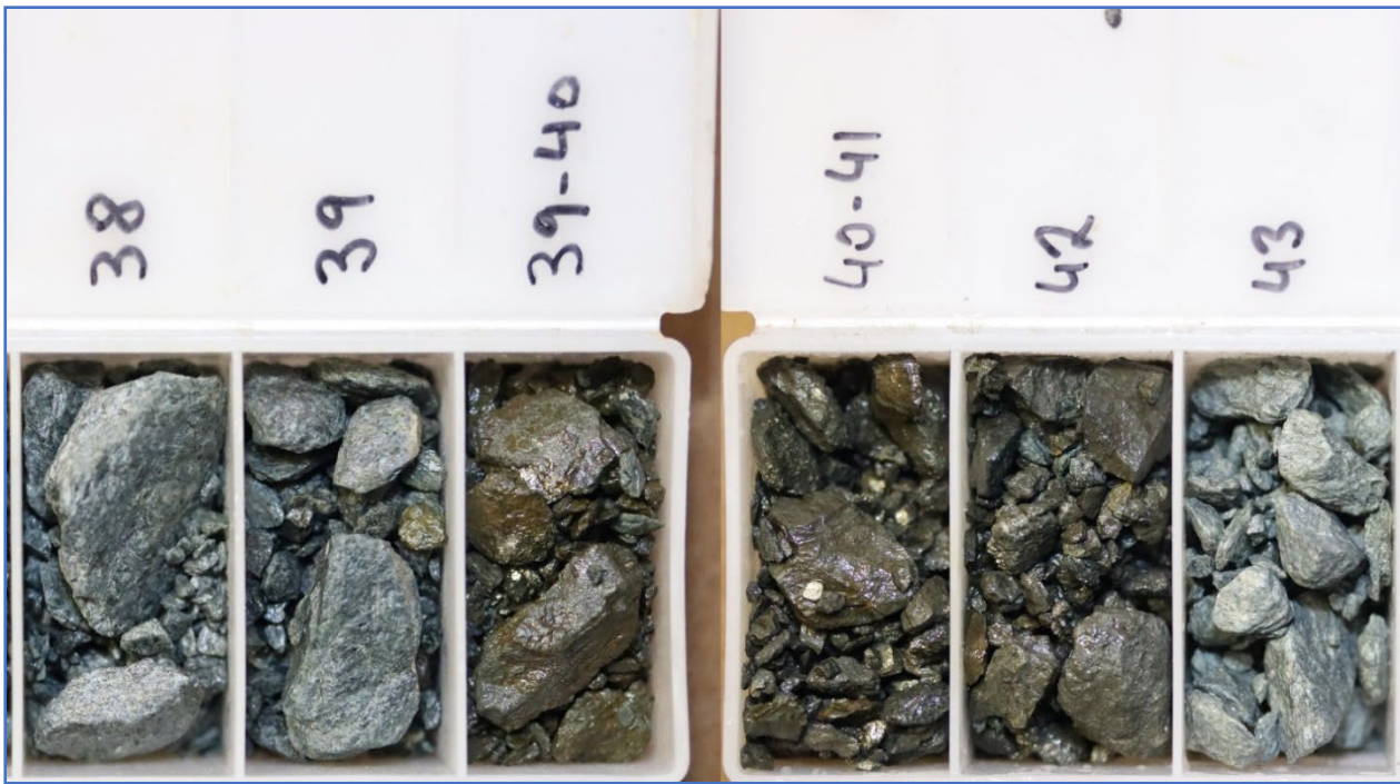
Figure 6: Visually logged chips from 23NRC009 showing massive pyrrhotite and pyrite from 39-42m *
