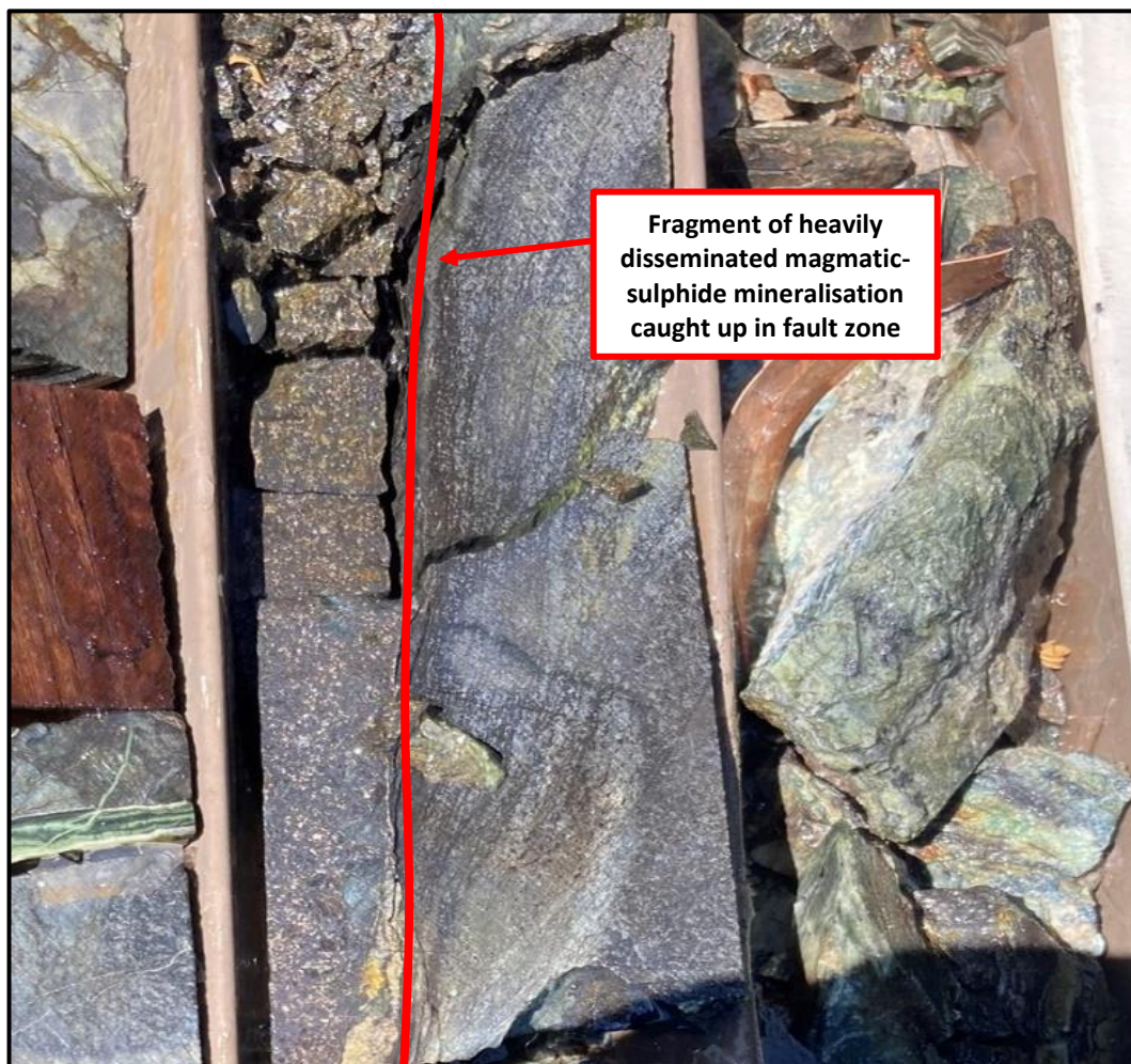
Photo One: Heavily disseminated magmatic-sulphide mineralisation in hole PS053
