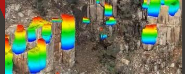
3D model of cliff face depicting the calculated 2,000 tonnes of dolerite rock removed.
