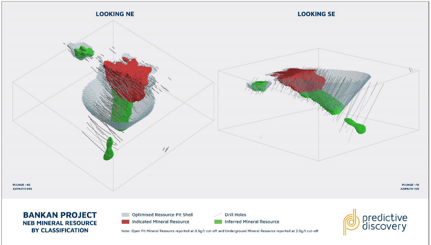
Figure 3: NEB block model showing the Indicated (red) and Inferred (green) Mineral Resource categories and drill traces. Left image looking north-east and right image looking south-east.
