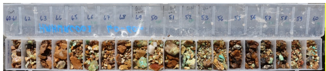
Figure 1. Chip tray from HMHWRC001: 40-60m showing malachite (Cu oxide). Laboratory analyses of this interval averaged 0.88% Cu with maximum value of 2.11% Cu between 54m and 55m.
