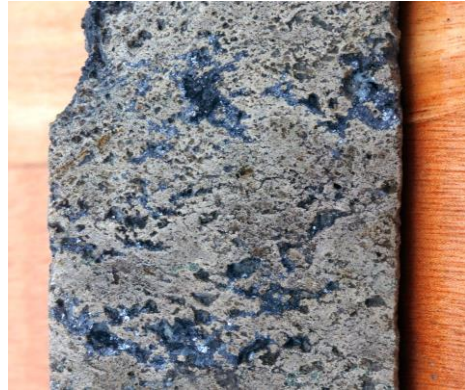
Structurally-related massive sphalerite and galena at TP13 from 3m 55% Zn+Pb
