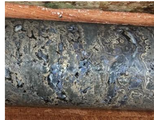
Concentric textured sphalerite and coarse galena within a breccia unit
