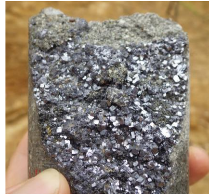
Fracture-fill coarse galena within sandstone unit
