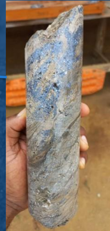
Massive galena and sphalerite in interpreted sheared system (NKDD026)
