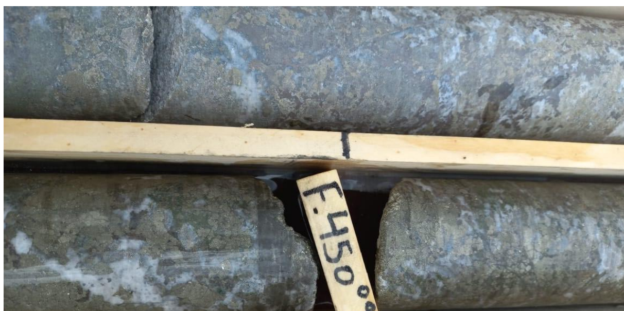
Image 1: GNDD-790 (Central Verde at depth) skarn alteration and sulphides logged (assays pending)
