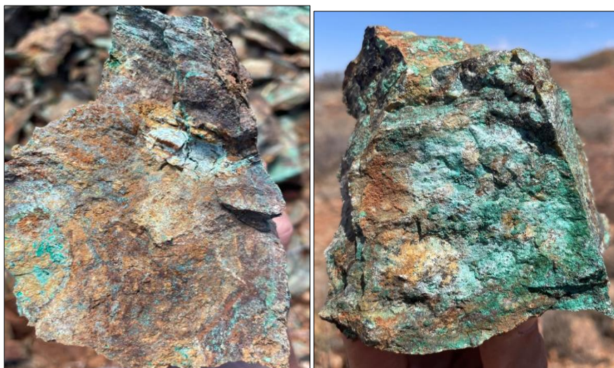
Figure 1 Samples from Bonya West. Left : Photo of rock chip sample JE0176 with 19.35% Cu; Right : Photo of rock chip sample JE0171 (that appeared on page 1 of the 9 November 2022 ASX announcement) with 1.55% Cu. The visual comparison is of interest, with the least superficially mineralised of the two, an order of magnitude more enriched.
