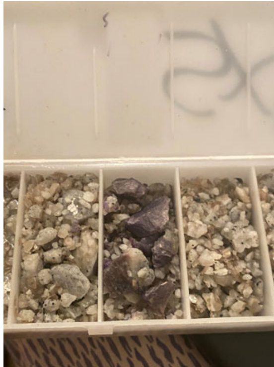
Figure 3 : Sieved samples presented in chip trays 185m - 186m downhole in SXRC0017, showing strong eucryptite mineralisation
