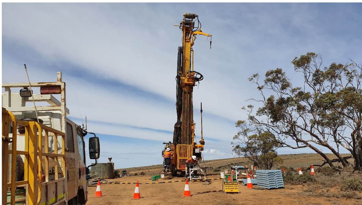
Figure 2. Drilling contractors undertaking metallurgical sample drilling at Iron Peak
