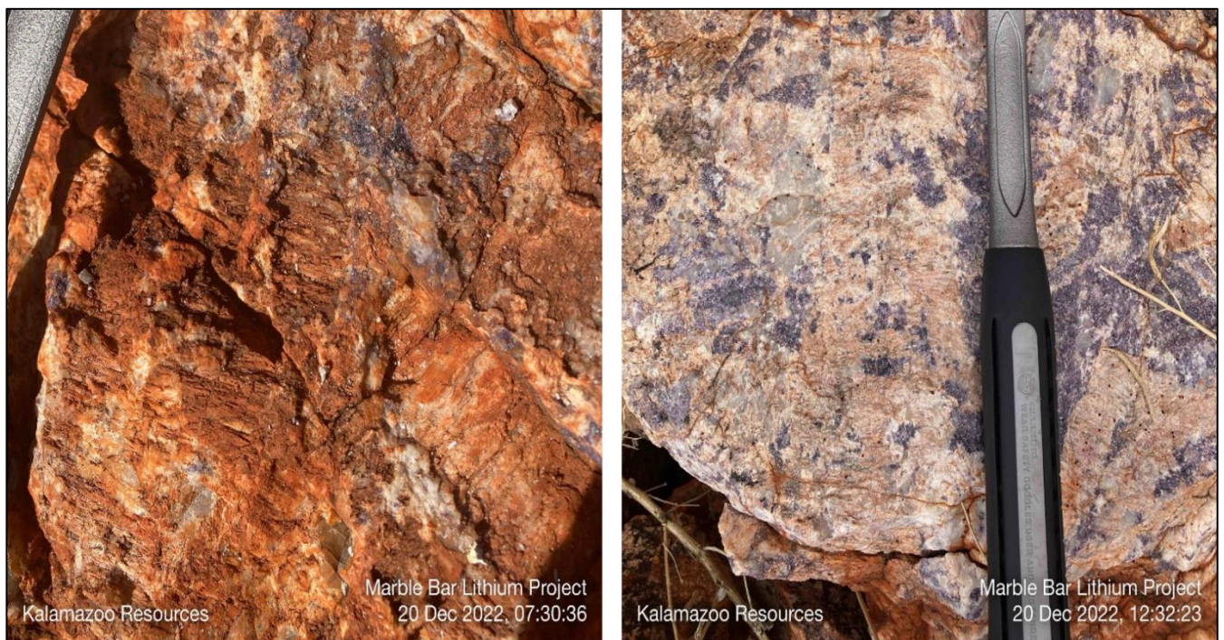
Figure 3: Example photos of spodumene (pale pink-white, coarse elongated striated mineral) and lepidolite (purple) mineralised pegmatite dyke in E45/5970, Marble Bar Lithium Project, East Pilbara WA. Note these photos correspond to rock chip sample MBLR212 which assayed 2.8% Li 2 O (see Table 1). Scale of view is ~40cm.
