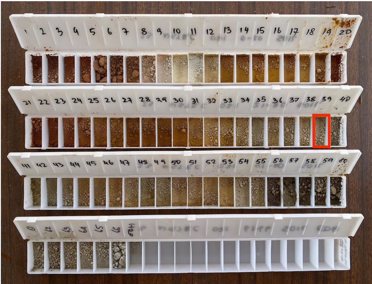
Figure 1. Reverse Circulation core samples from NSTRC071 showing weathering variation REE enriched regolith at North Stanmore. Note the interval between 39-40m with 1.08% TREO highlighted in Red.
