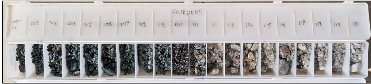
Figure 5: FGIR0005 chip trays showing 10m of pegmatite from 110m
