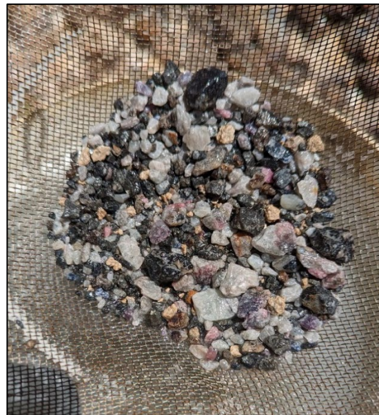
Figure 7: Rubellite and lepidolite bearing pegmatite (with lesser mafic material) in FGER0010 at 88m depth
