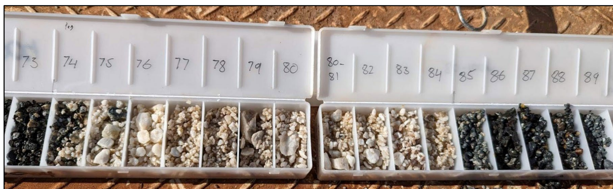
Figure 4: FGIR0004 chip trays showing 11m of pegmatite from 73m
