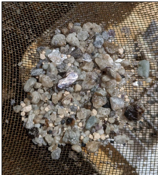
Figure 6: Lepidolite and cookeite bearing pegmatite in FGER0007 at 59m depth
