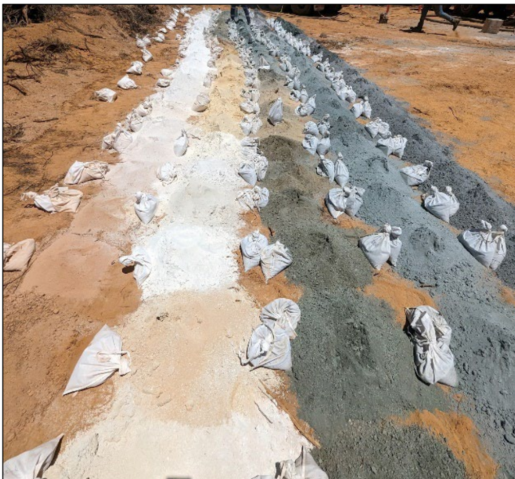
Figure 3A: Drill spoils from FSIR0003 showing felsic material over 32m
