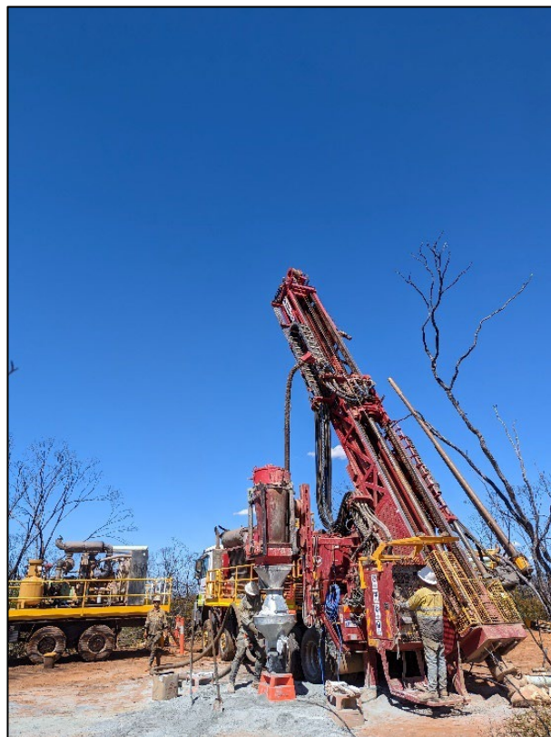
Figure 1: RC drill rig drilling at the South Iron Cap East Prospect
