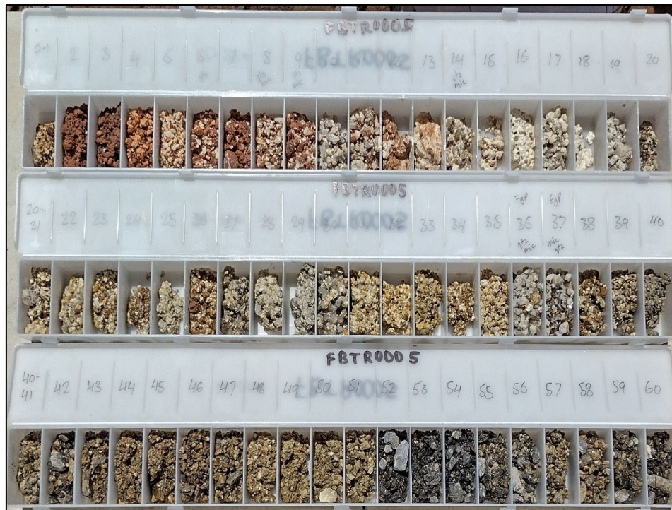
Figure 8: FBTR0005 where material from 7 – 21m was interpreted as highly weathered pegmatite with quartz, white clay and trace muscovite. Pegmatite also logged from 35 – 37m
