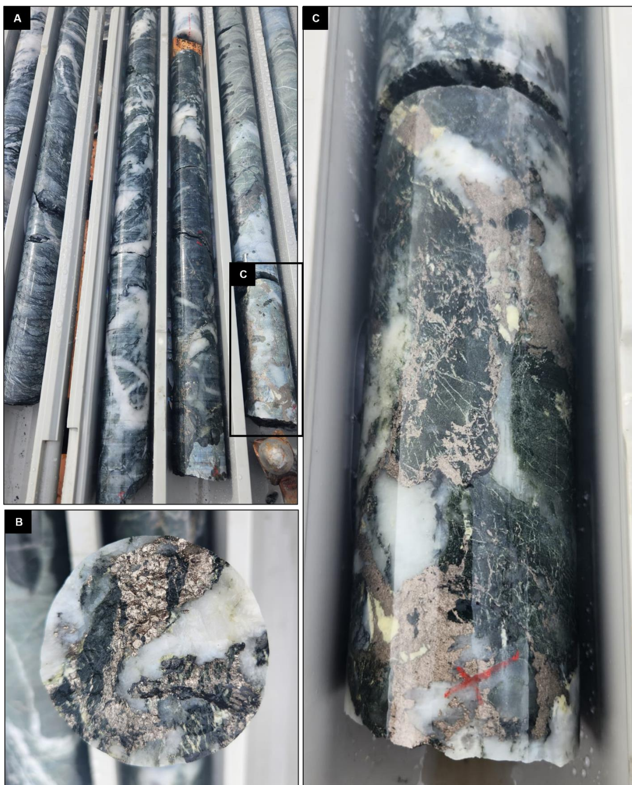
Figure 6 Core photographs and stockwork mineralisation 23LMDD01 intercept zone SW1.
