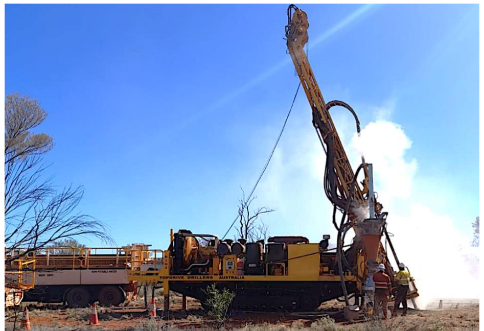
Figure 1: Track mounted reverse circulation drill rig used for Matilda South drilling.
