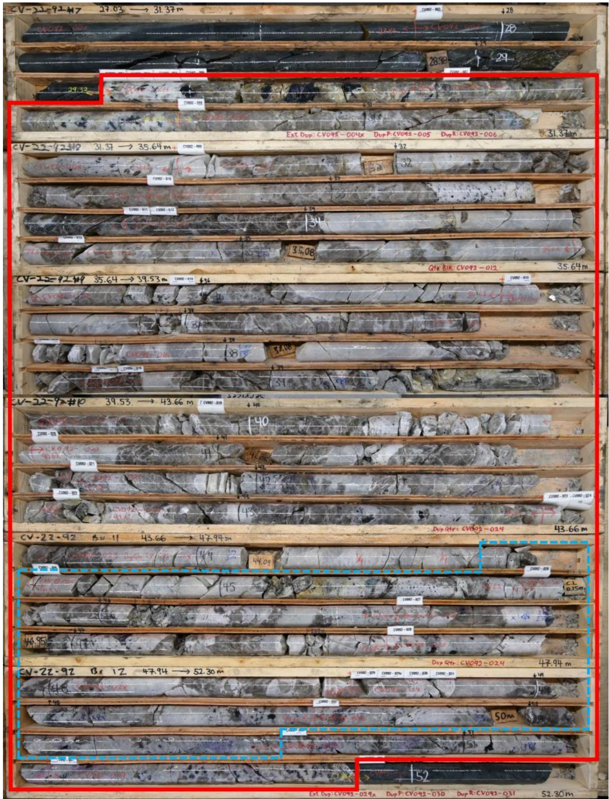
Figure 3: Spodumene drill-core intersection in drill hole CV22-092 (22.6 m at 1.56% Li 2 O, including 6.0 m at 3.19% Li 2 O)
