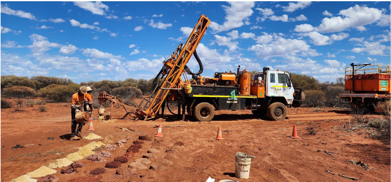
Plate 1 – Aircore Drilling in progress in unexplored areas east of Apollo Hill.
