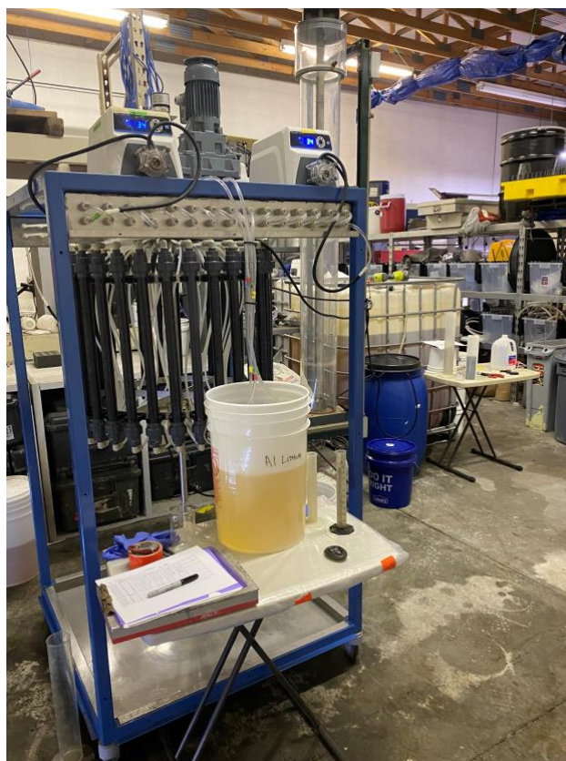
Figure 1: The benchtop Direct Lithium Extraction (DLE) setup in the independent laboratory in Salt Lake City
