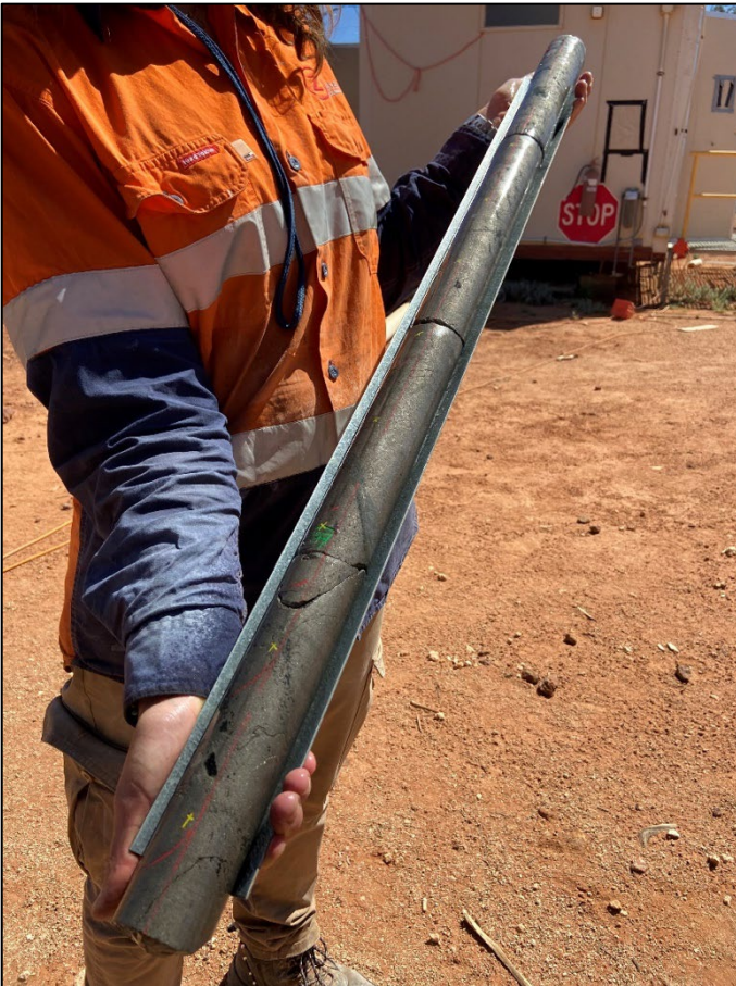
Figure 1: Example of diamond drill core of massive Ni-sulphide intersected in TED54, the third hole drilled at the Dimma Discovery, positioned above the discovery hole, TED41. The section of core in the photograph is approximately 1.0m long and starts from 196.75m downhole. See text for further details.
