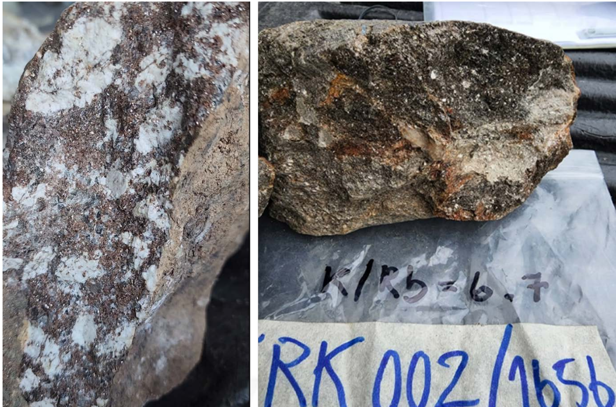
Photos: Polyolithionite (dark minerals, refer Appendix 1) in feldspar-quartz pegmatite float samples at Kanchanaburi
