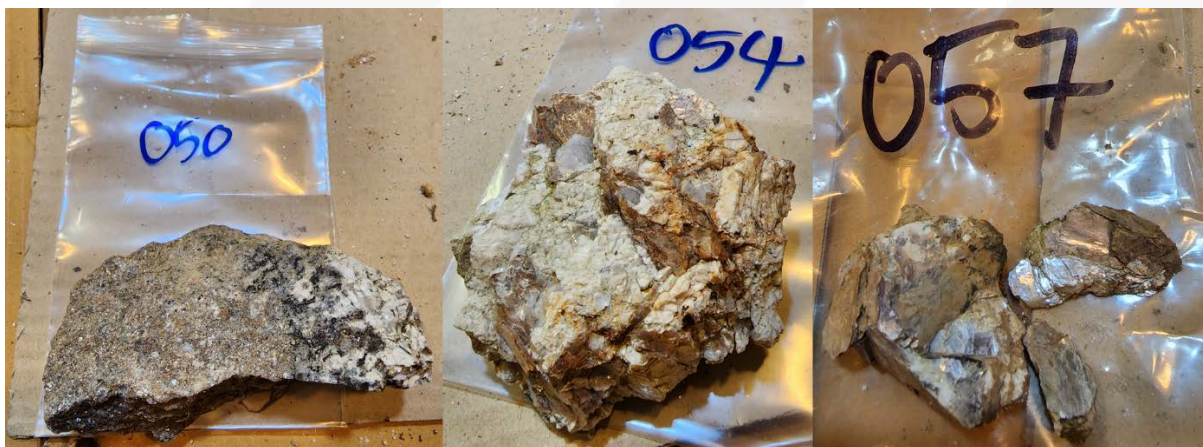
Photos: polyolithionite in pegmatite sample 050 (left), lepidolite pegmatite sample 054 (middle) and coarse lepidolite flakes 057 (right)
