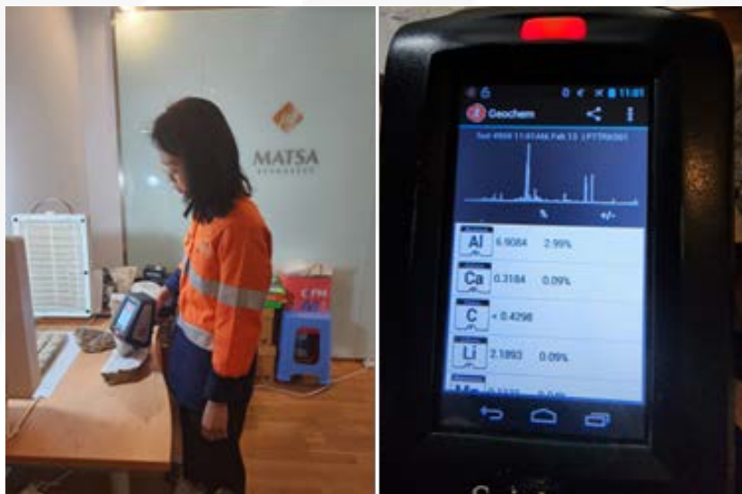
Testing a polyolithionite pegmatite sample (RATRK010) from Ratchaburi at Matsa's Bangkok office for lithium percent using LIBS analyser which in this instance, returned a reading of 2.19% Li (4.71% Li 2 O)
