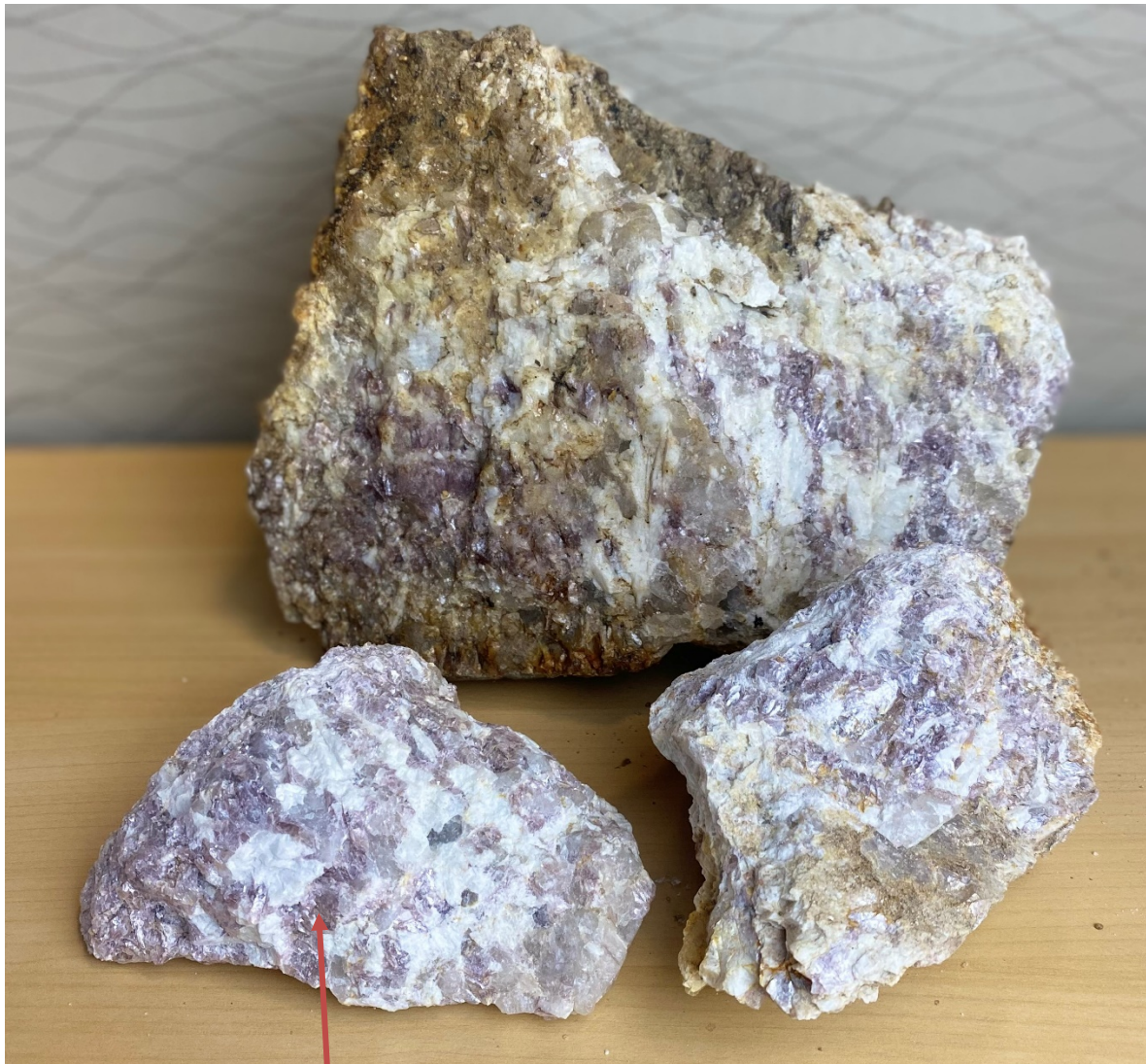
Photo: Rock samples from Pink Panther (Kanchanaburi) where LIBS analyser testing confirmed 3.45% Li (7.4% Li 2 O) in lepidolite bearing pegmatites
