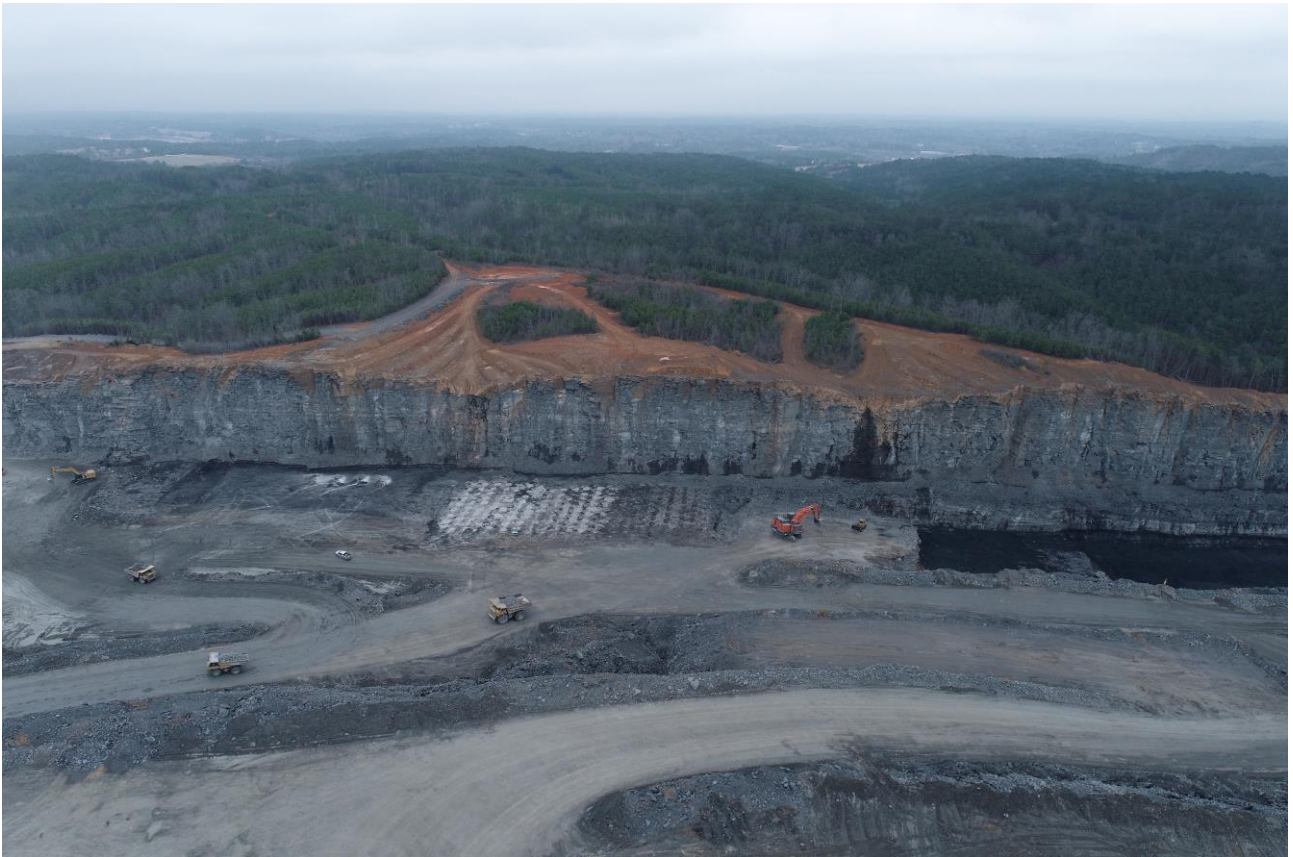
Image: Aerial shot of Black Warrior with Ex3600 in orange and CAT390 in yellow on far left – Newcastle seam bench on left and Mary Lee seam bench on the right
