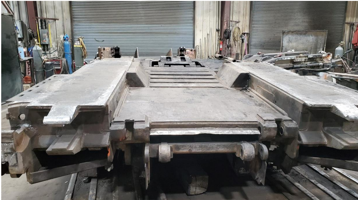
Image: CM06 from New Elk Mine and an overhaul workshop at Delta, Colorado – major components sandblasted and repaired ready for re-assembly
