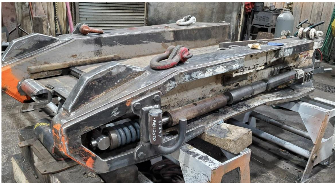
Image: CM06 conveyor tailpiece re-worked and re-assembled at the Delta workshop
