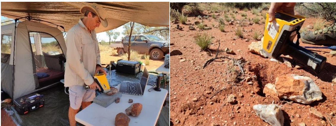
Figure 4 and 5: Portable XRF was utilised to assess individual rock samples and map areas of enhanced prospectivity for follow-up geophysics surveys.
