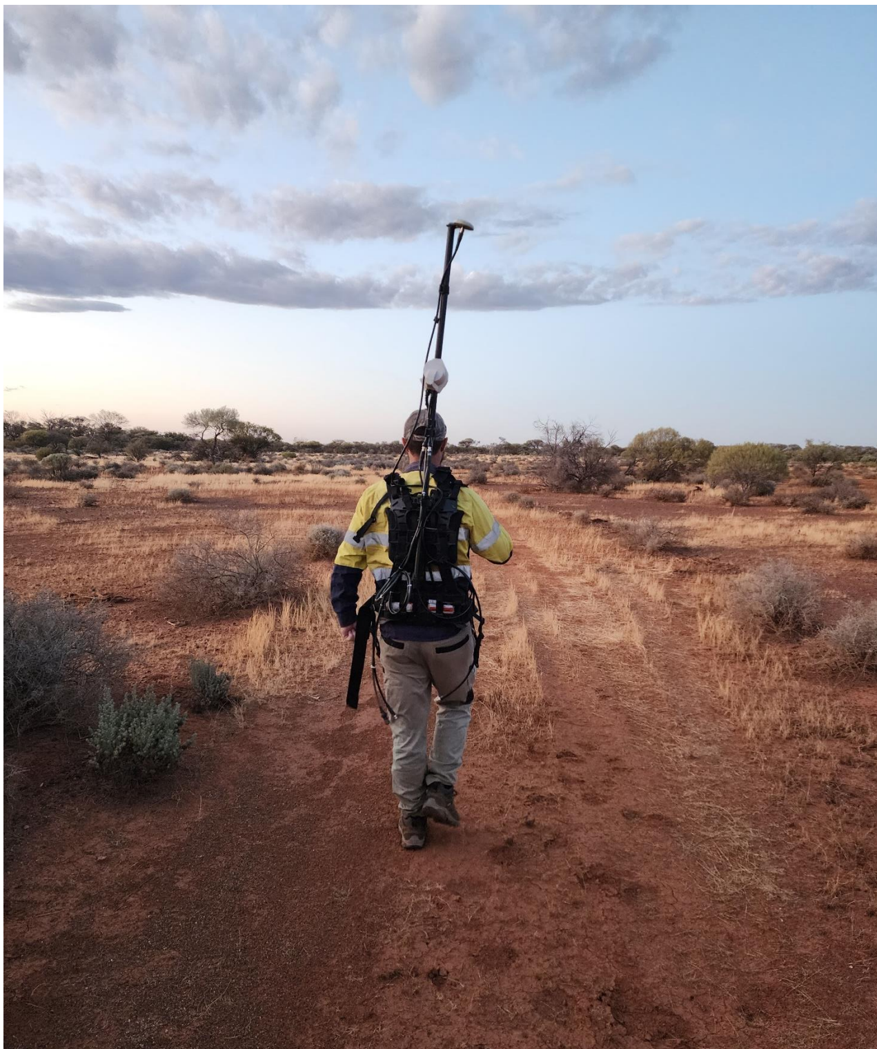
Figure 1; Ground magnetic survey data acquisition by field crew at the Canegrass Battery Minerals Project.
