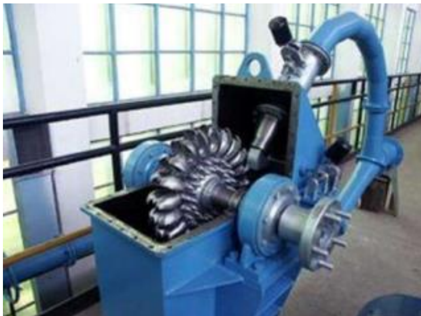
Figure 1: Example of commercially available Small Pit Pelton hydro power unit for location at the recovery site
