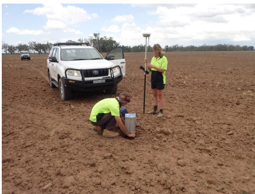
Figure 3. Photograph of contractors from Fender Geophysics employing a Scintrex CG5 gravity meter to take readings at the Myall Project.
