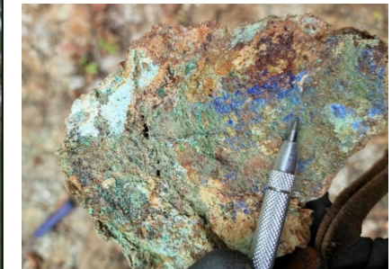
Hand specimen displaying azurite and malachite copper oxide mineralisation
