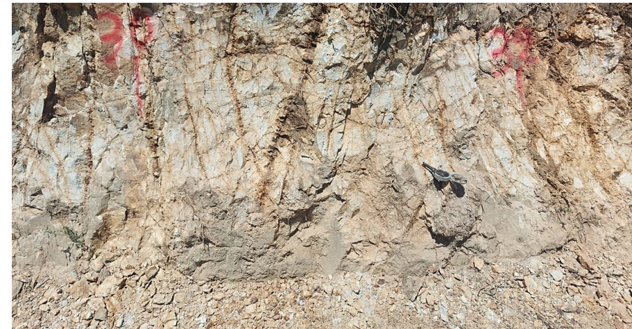
Barbasco Guayacan Prospect: Quartz diorite porphyry, stockwork of B and D veins, Channel Sample HTC015: 44m@ 0.21 g/t Au and 0.18% Cu
