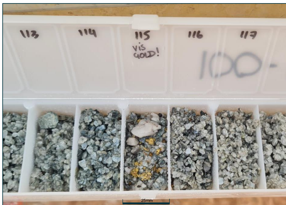
FIGURE 3: 23MBRC006A CHIP TRAY SHOWING 112 TO 117M DOWN HOLE
