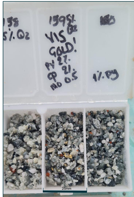
FIGURE 2: THE SECOND INTERSECTION OF COARSE VISIBLE GOLD IN 23MBRC006A FROM 158 TO 159M.
