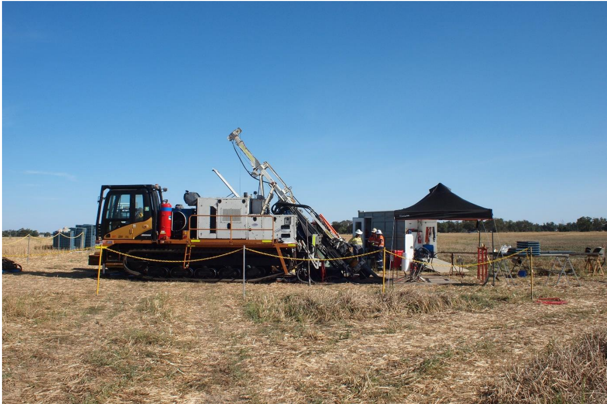
Figure 3 Diamond drill rig at the Ironbark East Prospect
