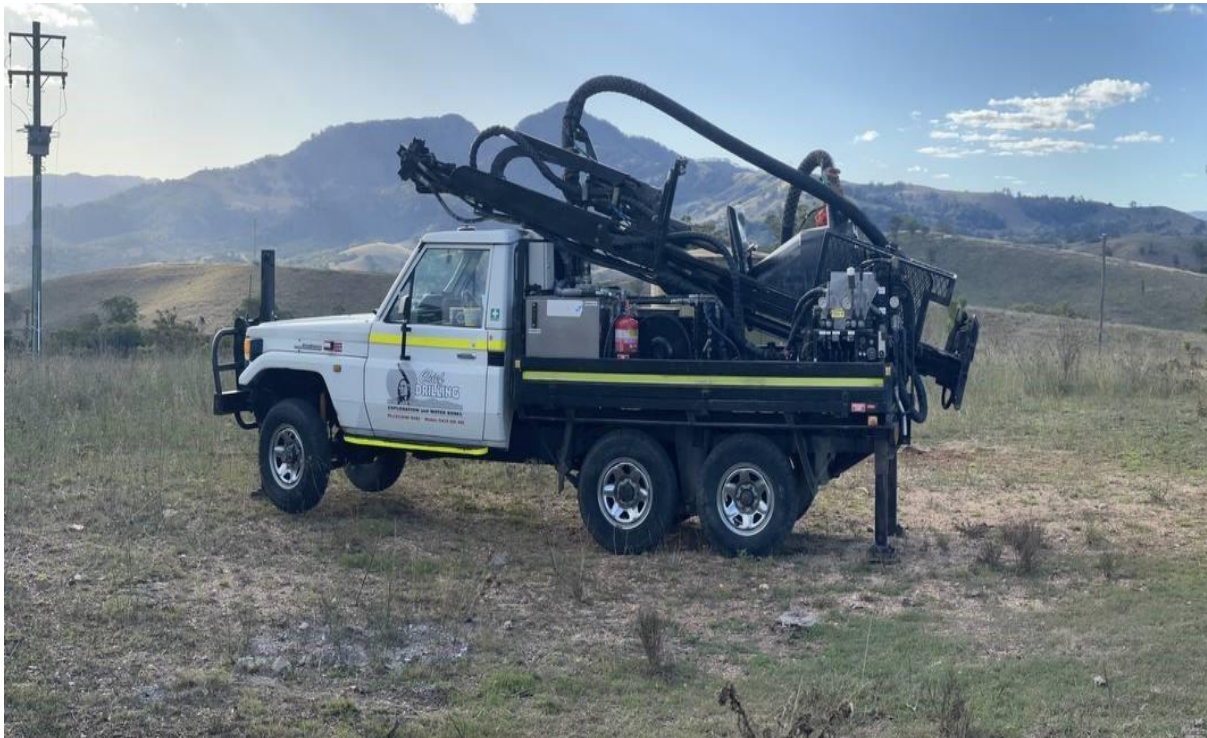
Figure 2. Aircore drill rig at EL8944
