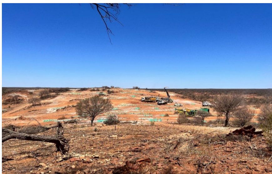
Plate 1 – Cleared area over bulk sample pit location at Apollo Hill. View looking South. A 5,000m RC grade control drill program is in progress. Diamond drill rig completing additional metallurgical sample drilling and geotechnical drilling also in shot. Photo taken 17 February 2023.
