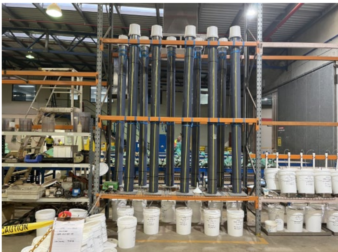
Plate 2 – Column leach optimisation work underway in the laboratory.
