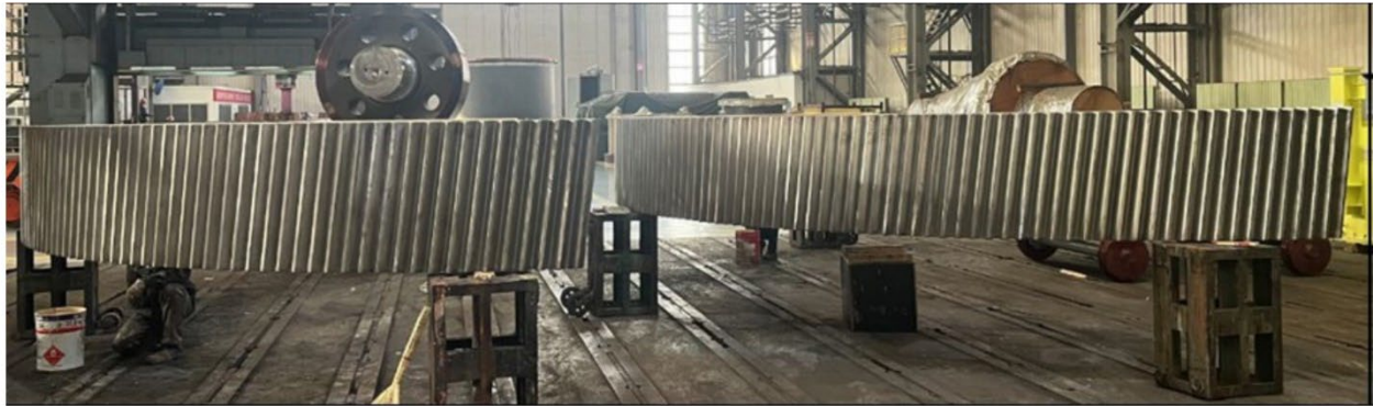
Figures 4-6: Top – Mill girth gear, shell section and shell end. Mill fabrication well advanced for delivery to site ahead of schedule in March 2023.
