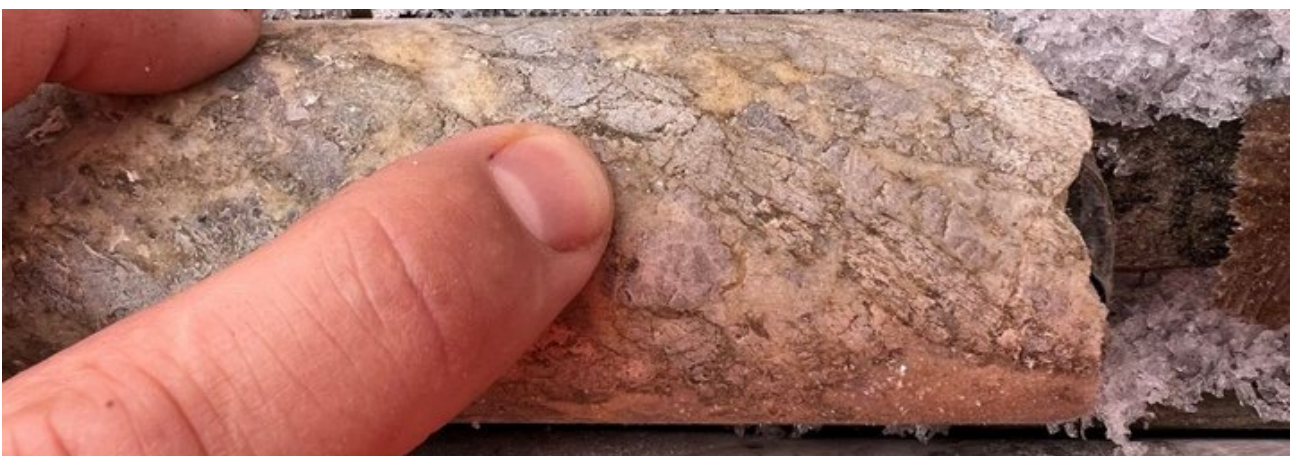
Figure 1: Visible spodumene observed in drillcore from AC-2010-004 between 212.8m and 223.8m. NO historic drill core has ever been assayed for Lithium bearing minerals.
