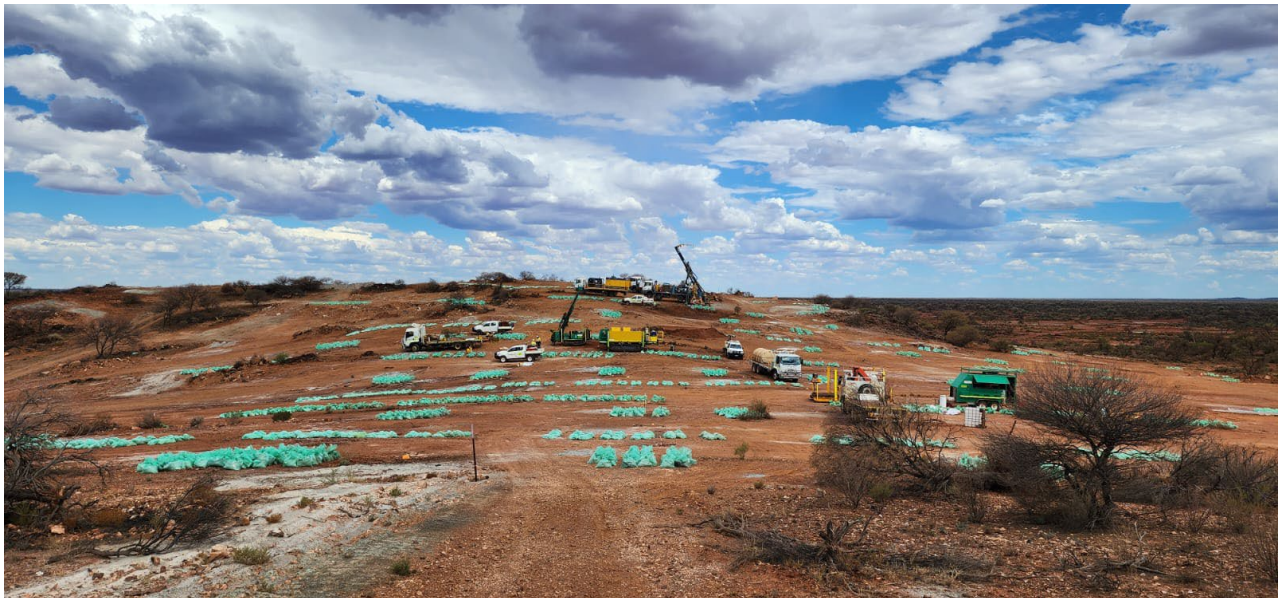
Plate 1 – RC grade control and geotechnical diamond drilling in progress at Saturn’s planned Apollo Hill bulk sample pit location. Photo taken 21 February 2023.
