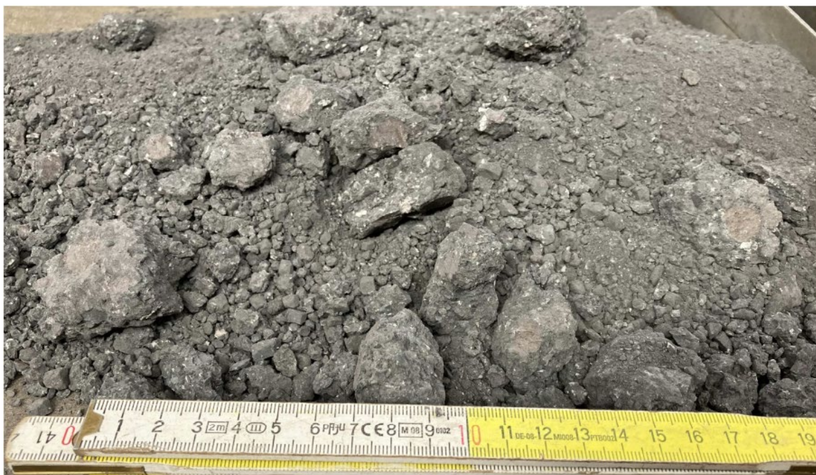
Figure 9: High Pressure Grinding Roll (HPGR) test discharge material (Razorback 'adit' bulk sample)
