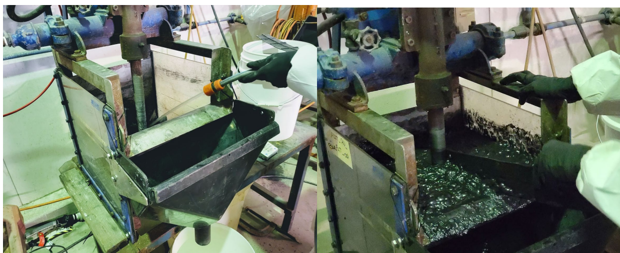
Figure 12: Laboratory 30 litre Agitair froth flotation cell used for bulk flotation work (left), and Razorback 'adit' sample flotation test in progress (right). Froth, containing gangue silica-rich waste material is removed, concentrating iron-rich minerals in the remaining sample.
