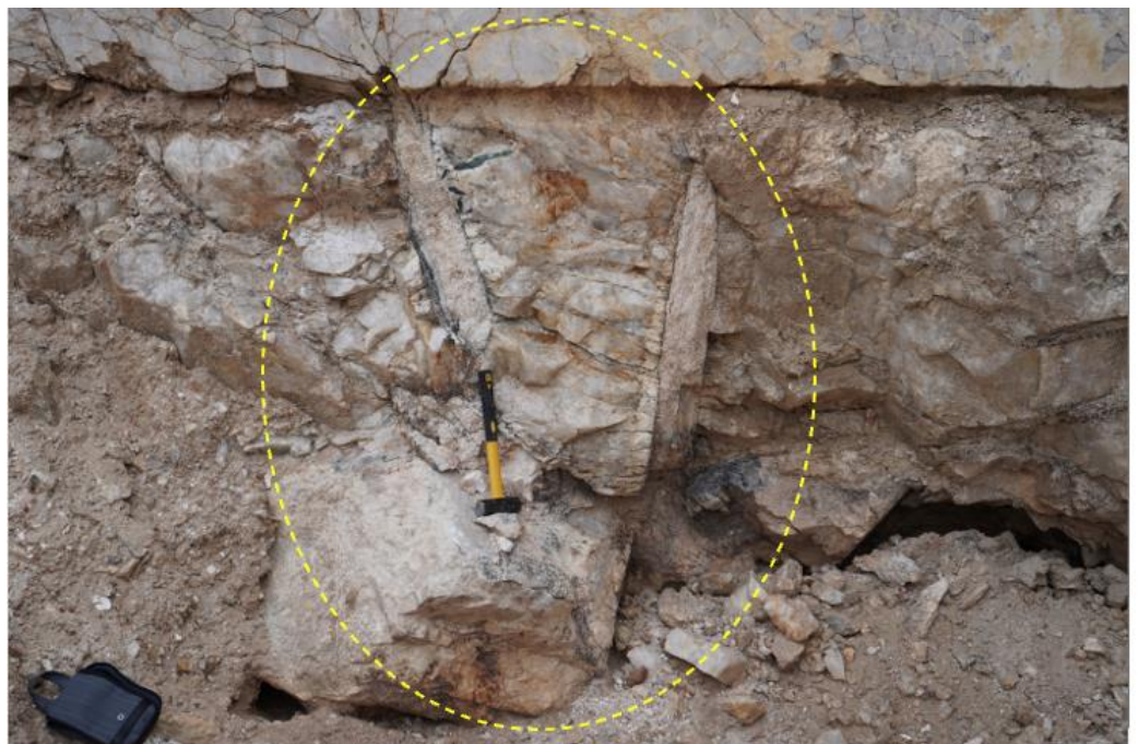
In-situ weathered spodumene crystals in the Mina Bom Jesus de Baixo pit
